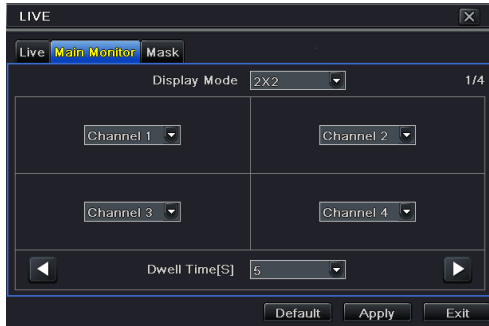
Fig 4-8 Live Configuration-Main Monitor
