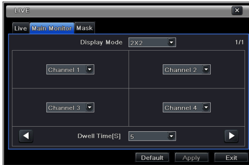
Fig 5-7 Live Configuration-Main Monitor
